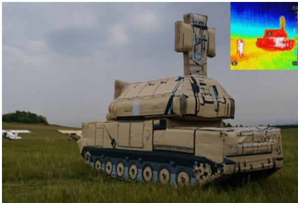
Figure 12: Electromagnetic Emitter Installed in A Modern Decoy
